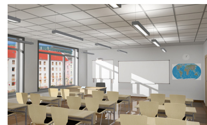
Morning: sensors dim the lighting to utilise daylight and save energy
