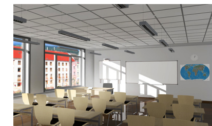
Break time: switching off lights automatically when the classroom is empty can reach up to 50% savings
